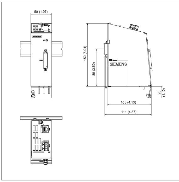
Figure 18-13 Dimension drawing of the SMC20
