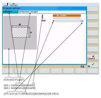
Figure 8-38 Screen for user cycle CYCLE67 and code for CYCLES67 in "sc.com"
