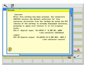
Figure 10-16 Line contactor message text
