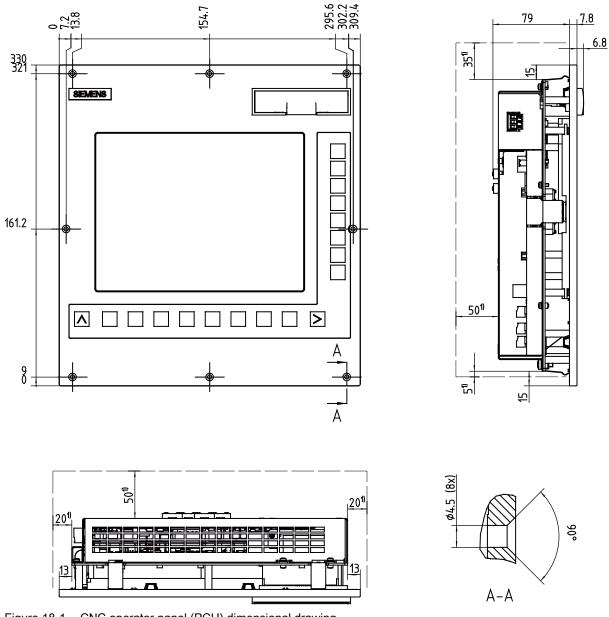
Figure 18-1 CNC operator panel (PCU) dimensional drawing
