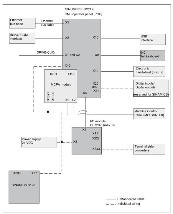
Figure 5-3 Connection overview with MCPA module
