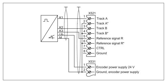
Figure 2-16 Connection example 2: HTL encoder, unipolar, with reference signal<sup>1)</sup>
