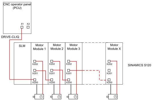
Figure 5-10 Connection with SLM (Smart Line Module) and DRIVE-CLiQ
