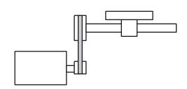
The axis can now be traversed. The direction of movement can be reversed with MD32100  $MA_AX_MOTION_DIR = 1 \text{ or } -1$  (without affecting the control direction of the position control).
