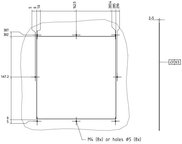
Figure 18-3 CNC operator panel (PCU) hole drilling template
