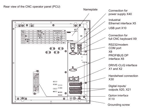
Figure 1-4 Position of the interfaces and front elements on the CNC operator panel (PCU)
