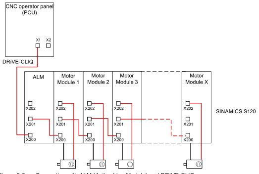
Figure 5-9 Connection with ALM (Active Line Module) and DRIVE-CLiQ
