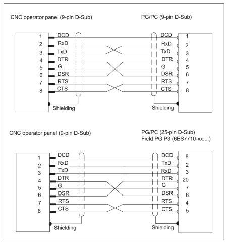
Figure 5-4 Connection diagram for interconnecting the CNC operator panel and the PG/PC
