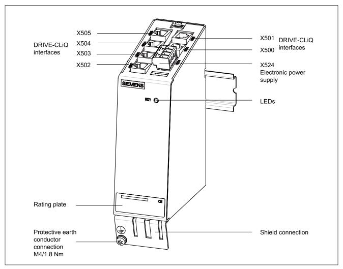
Figure 2-11 Interface description of the DMC20
