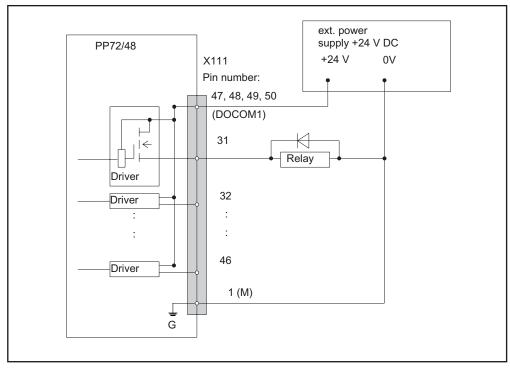
Figure 2-9 Terminal assignment for the digital outputs
