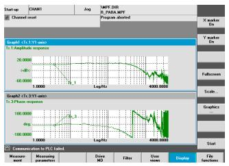
Figure 11-8 Optimized speed control loop
