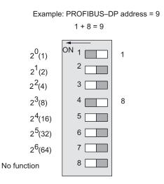
Figure 8-53 Setting the PROFIBUS-DP address on PP72/48
