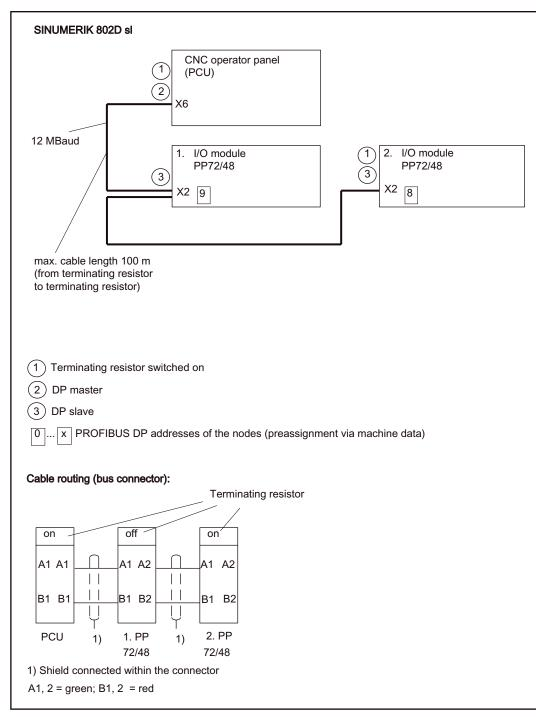
The diagram below shows a networking example for SINUMERIK 802D sl with two PP72/48 I/O modules.
