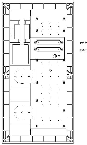
Figure 2-3 Interfaces at the MCP 802D sl
