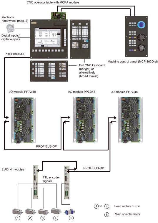
Figure 1-3 System overview with ADI4 (example configuration)
