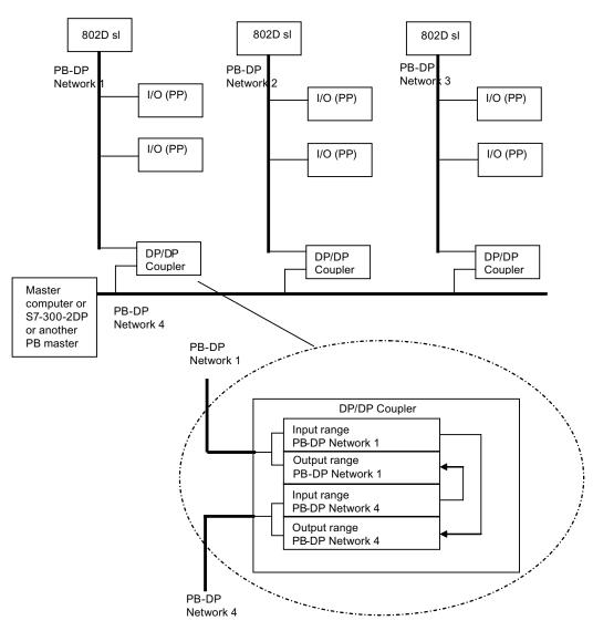
Figure 5-8 Using DP-DP coupler (example)
