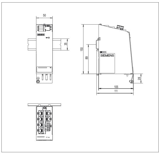
Figure 18-11 Dimension drawing of the DMC20
