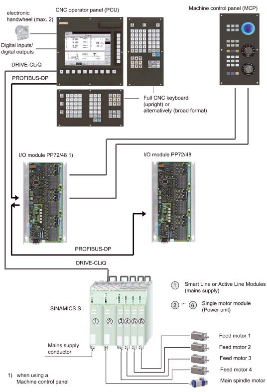
Figure 1-1 SINUMERIK 802D sl with SINAMICS S120 (example configuration)
