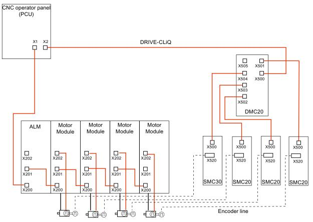
Figure 5-11 Connecting the DMC20
