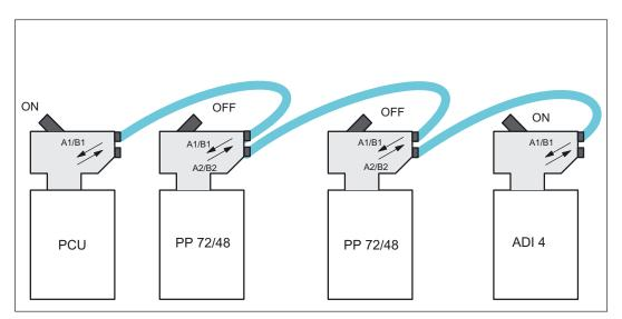
Figure 5-5 Basic arrangement of a PROFIBUS line
