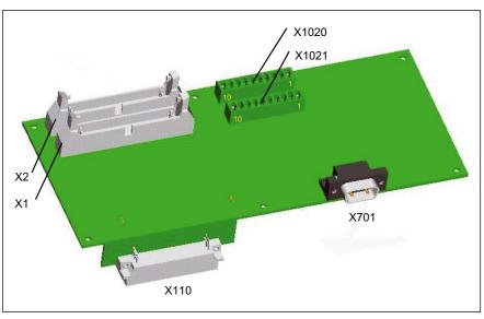
Figure 2-5 Position of the interfaces on the MCPA module
