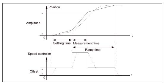
Figure 11-10 Signal chart for position setpoint/ramp measuring function
