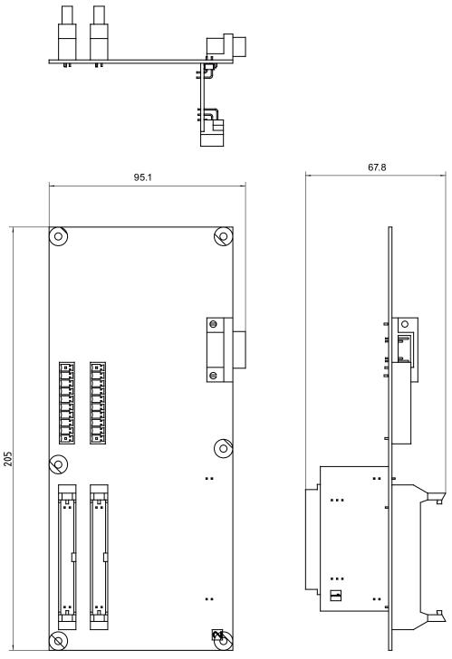
Figure 18-9 Dimensional drawing MCPA module
