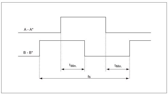
Figure 17-2 Signal characteristic of the A and B track between two edges: Time between two edges with pulse encoders
