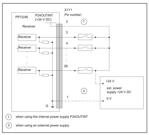
Figure 2-8 Terminal assignment for the digital inputs
