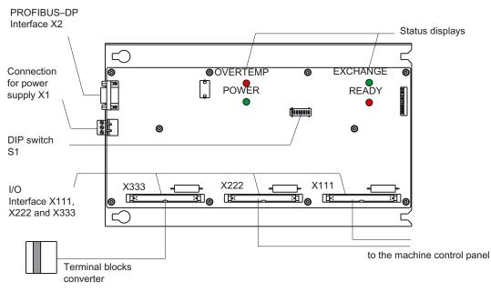
Figure 2-6 Position of the interfaces and status displays on the I/O module with connection to the MCP and a terminal strip converter
