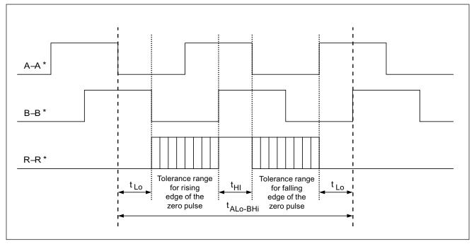
Figure 17-3 Position of the zero pulse to the track signals
