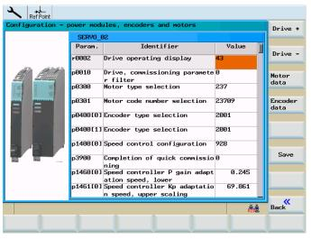
Figure 10-21 Configuration - Power units, encoders and motors
